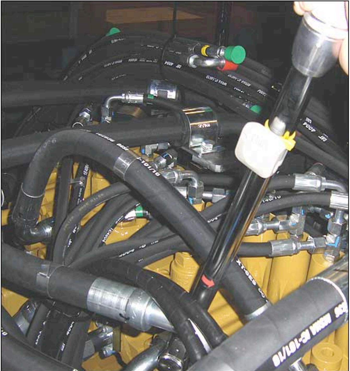
By placing an RFID tag on each wrench, Caterpillar knows that the proper tool—and, therefore, the correct amount of torque—was used.
