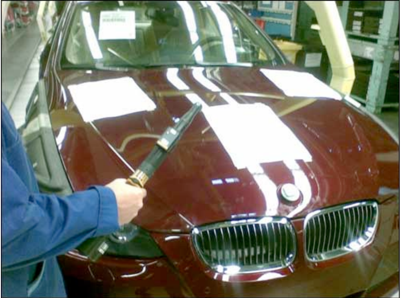
RFID tags attached to tools and vehicles make sure workers use the correct implement at the right setting.
